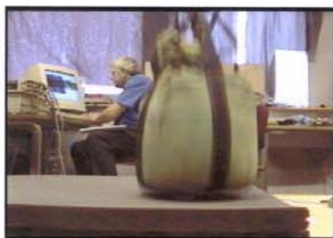
Figure 9: Video frame and pressure image of bagdrop
